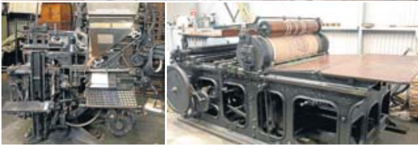
Two of the working machines on show at Penrith - a 1925 Model 8 Linotype and Wharfedale flatbed press.
