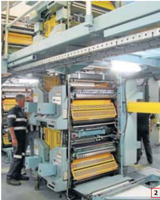
The new Tamworth press centre with reelstands from Wagga Wagga (1), a re-built tower showing yellow safety guards (2), one of the old Solna units (3), the Kodak CTP lines (4), and new press consoles (5).
